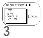
Press the PLAY/▲ button or the STOP/▼ button to select ON-TIME. Then, press the REW(ind)/◀ button or the F.FWD/▶ button to select your desired wake up time. Each press of the REW(ind)/◀ button or the F.FWD/▶ button will increase (or decrease) the time by 10 minutes.
